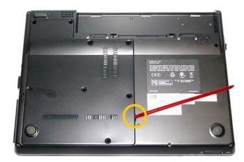
5. To remove the existing flash module, depending on the type of module you have, you must either pull up the module in the direction as shown in Figure 7, or remove the two screws as shown in Figure 8. Rock the module carefully until free of the connector.
